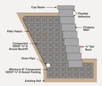
**Battered Gravity Retaining Wall**
