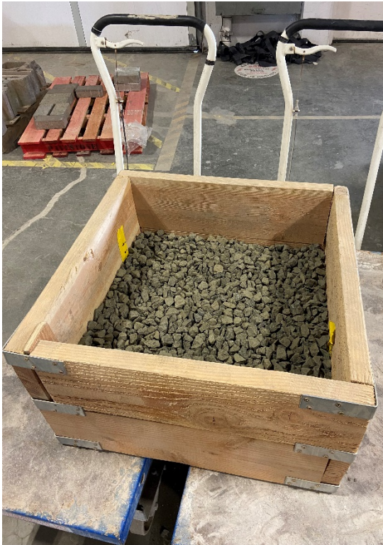
Photo #3 Frame with Upper Ballast Layer
