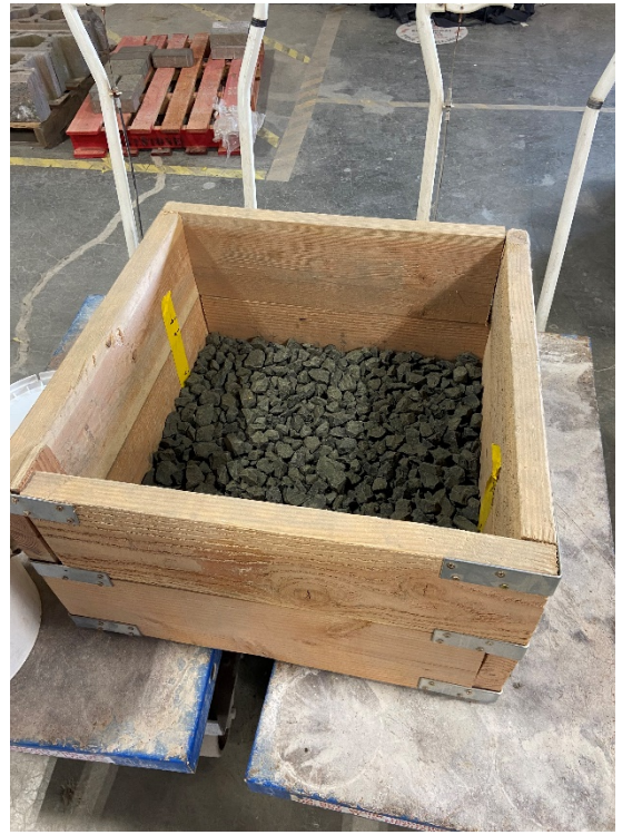
Photo #2 Frame with Lower Ballast Layer
