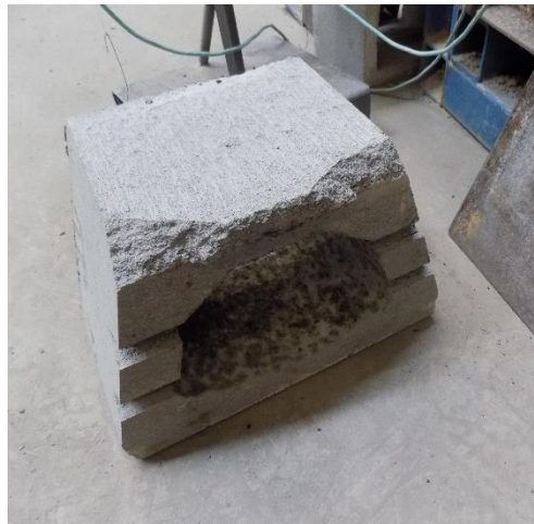
Figure 8 – Typical Failure Mode
