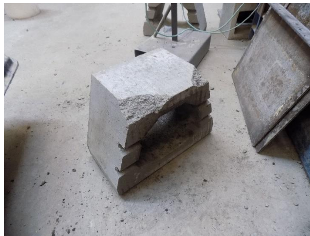
Figure 8 – Typical Failure Mode
