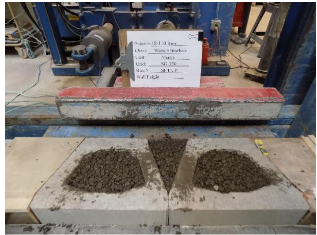
Figure 3 – Bottom Course with Compacted Aggregate
