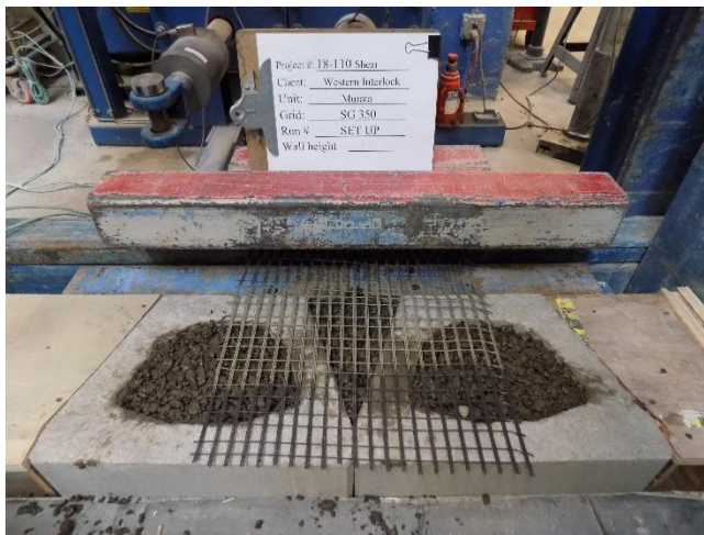
Figure 4 – Placement of Geosynthetic
