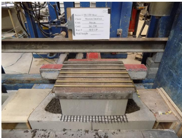
Figure 6 – Neoprene Pads, Loading Plates, and Beam
