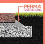
CLEAR/OPEN GRADE - ASTM No. 9 (leveling) - Compacted Base (3/4 inch)
