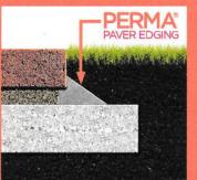
DENSE/CRUSHED BASE - Sand (leveling) - Compacted Base (0-3/4 inch)
