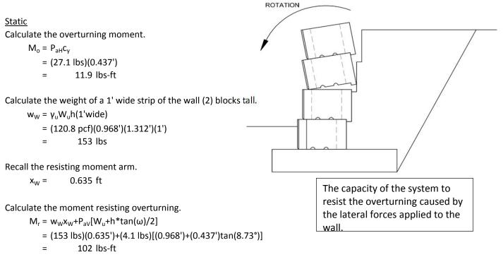
Calculate the factor of safety for the retaining wall overturning about the front corner of the (2) block.
