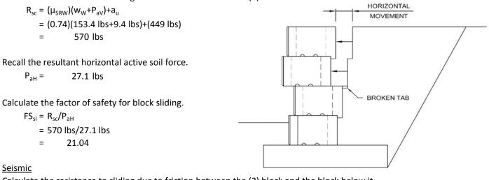
Calculate the resistance to sliding due to friction between the (2) block and the block below it.
