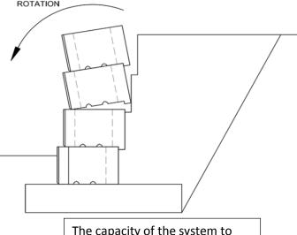
The capacity of the system to resist the overturning caused by the lateral forces applied to the wall.
