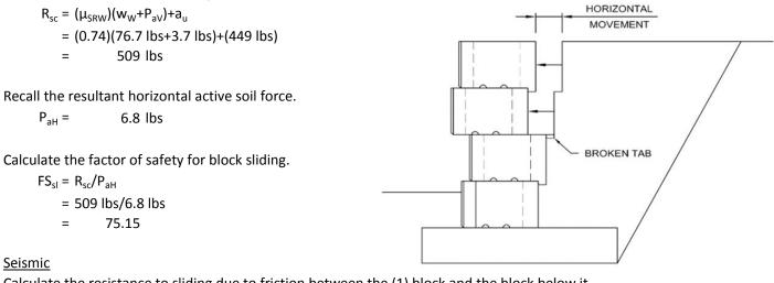
Calculate the resistance to sliding due to friction between the (1) block and the block below it.
