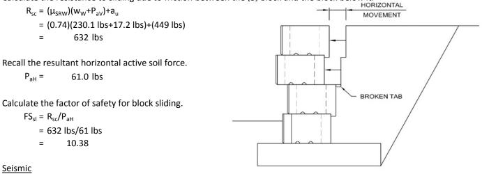
Calculate the resistance to sliding due to friction between the (3) block and the block below it.
