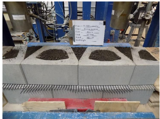
Figure 5 – Second Course of SRW Units with Aggregate
