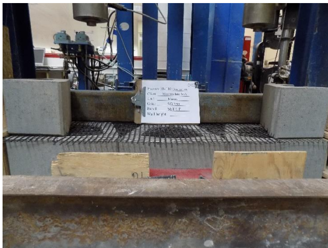
Figure 4 – Placement of Geosynthetic
