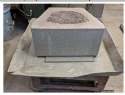
Photo 2: Hollow portion of block filled with aggregate and consolidated by a vibrating table operating for approximately 1 min. until no visual consolidation of aggregate was observed.
