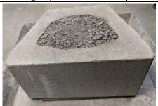
Photo 1: Hollow portion of block filled with aggregate by shoveling. No vibration was used.
