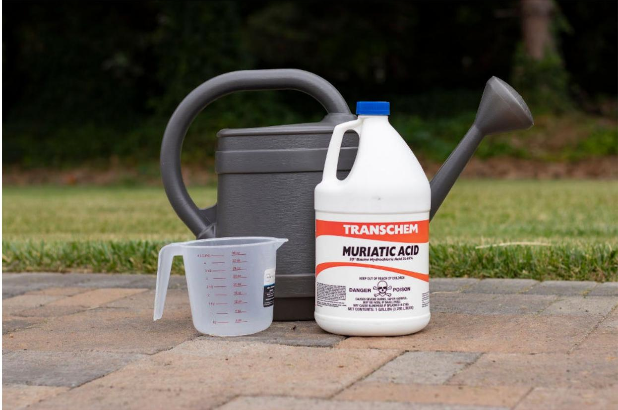
We recommend filling the water can first, then add your acid. We've found it helpful to use a cheap, plastic graduated measuring cup to help you measure and add in the Muriatic acid. If you don't, you'll risk overfilling the watering can and spilling the mixture.
