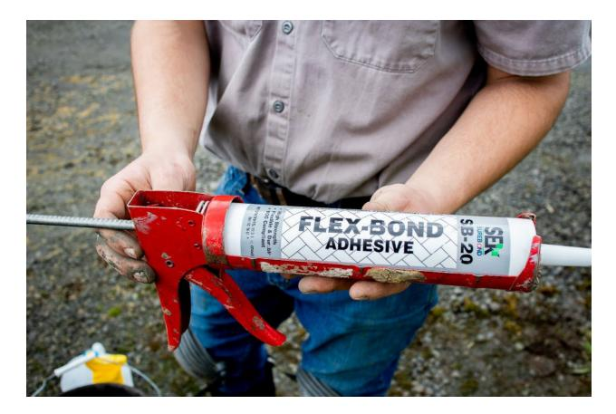
It's worth noting that we prefer beads because it's easier to avoid any drips or spillover on the sides of your column. Keeping your beads and dots at least 2" away from the outside edge of the block for Chateau also helps avoid glue from oozing onto the face of the block.
