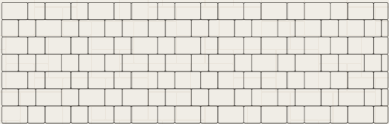
Two Stone Step Running Bond: Works with any stone that has more than one size it can module with (typical ratio 60% rectangles, 40% squares)
