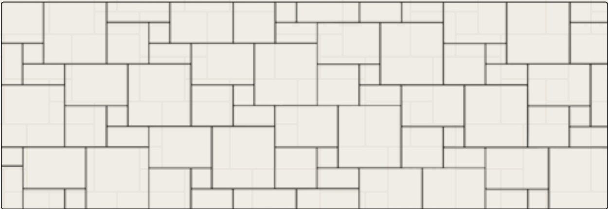
Five Stone Pattern: Works with Granite and Standard finish stones. 34% Arena, 26% Plaza, 20% Park, 11% Holland, 9% Half Holland
