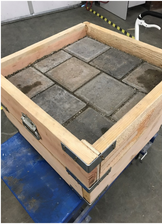
Photo #4 Running Bond as Installed
