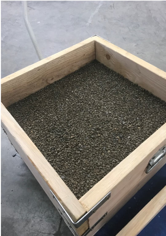
Photo #3 With Levelling Course
