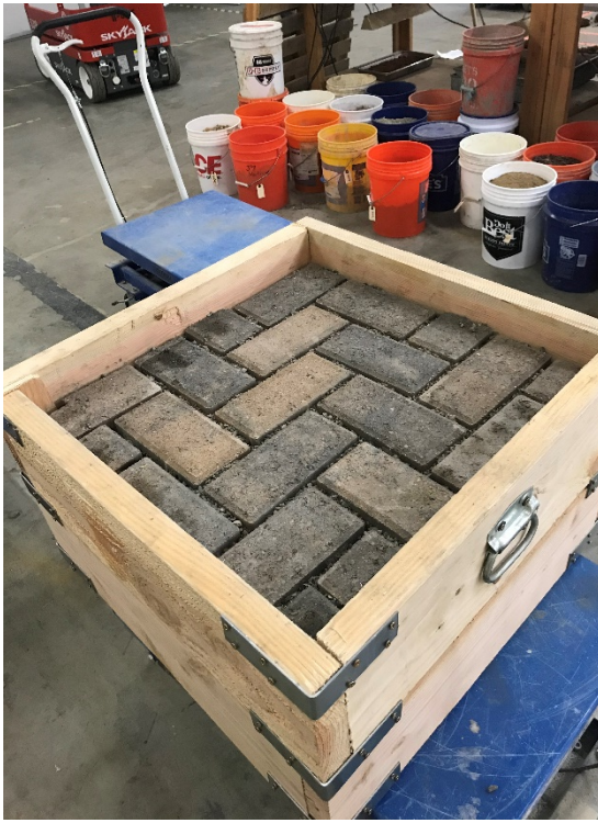
Photo #4 Herringbone as Installed
