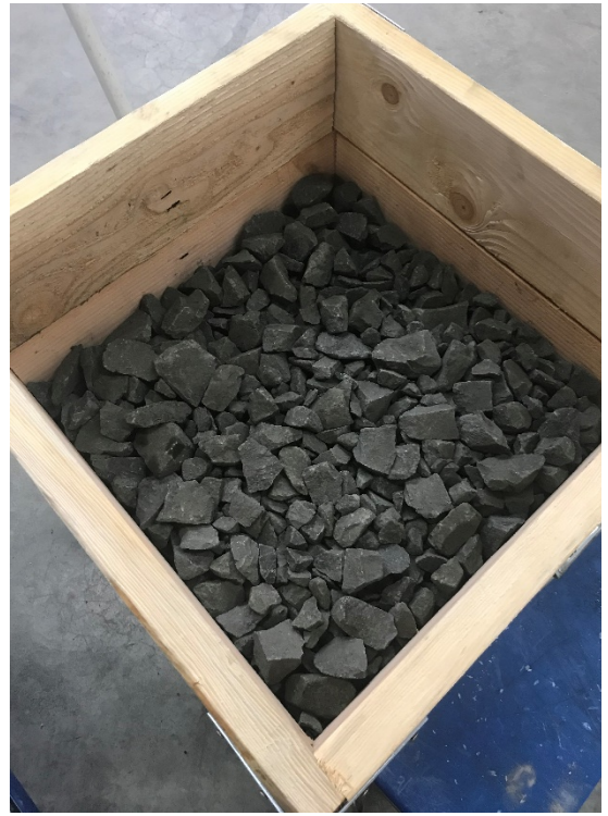
Photo #2 Frame with Ballast Layer
