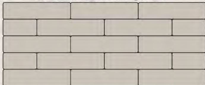
Running Bond: 100% 400mm blocks w/1 or 2 200mm block starter blocks per course
